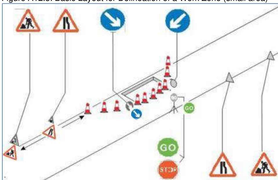
Figure A12.3: Basic Layout for Delineation of a Work Zone (small area)
